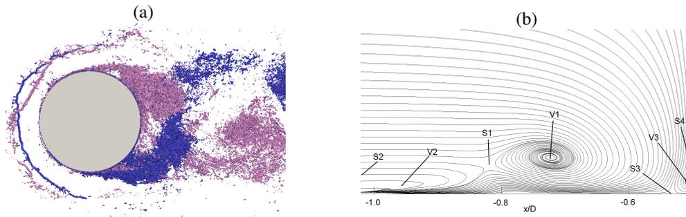
**Figure 1.** Overview of the flow field. Top view of isosurfaces of the Q-field at two instances in time (with different colours) (a) and streamlines of the time average velocity field in front of the cylinder (b).
