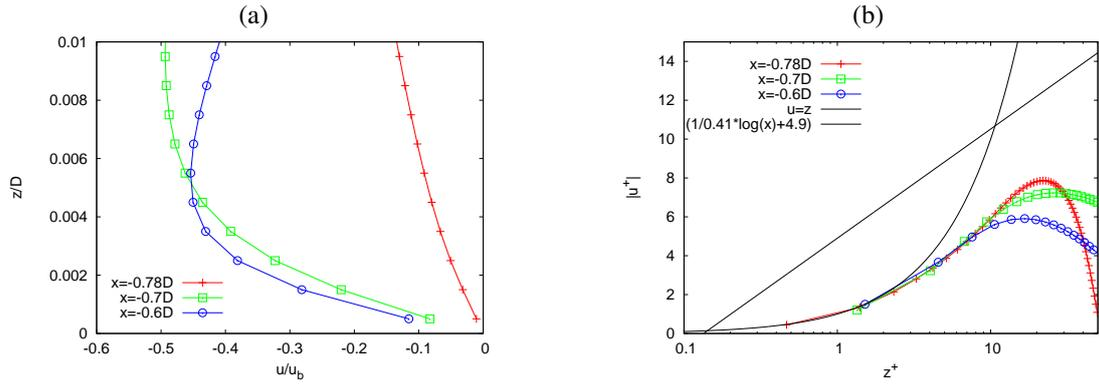
**Figure 2.** Velocity profile in the symmetry plane in front of the cylinder at three different positions of  $x$  in outer scaling (a) and in inner scaling (b).
