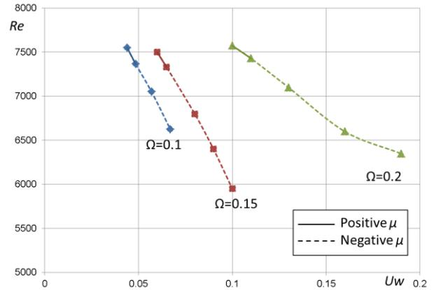
**Figure 3.** Variation of  $Re$  with  $U_w$ . This  $Re$  corresponds to the value occurring the exchange of the most unstable mode from the TS to the oblique TS.
