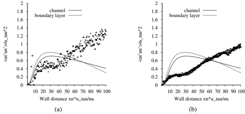
Figure 3: Reynolds shear stress of adjacent profiles in a coordinate system parallel to the wall ( $x_t, x_n$ ), expressed in inner coordinates at  $x/h = 8$  for  $Re = 37000$  (a) and  $Re = 10600$  (b).
