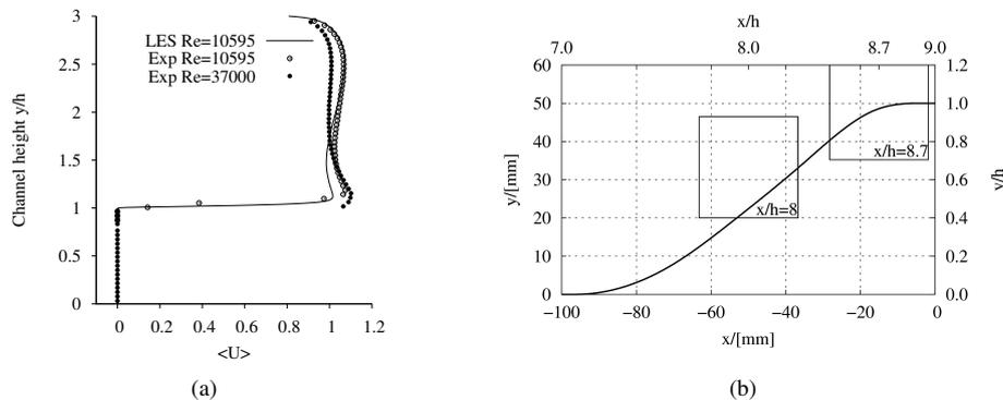
Figure 1: Comparison of the velocity distributions on the top of the hill, determined by previous PIV-measurements and LES (a). Positions of current measurements (b).
