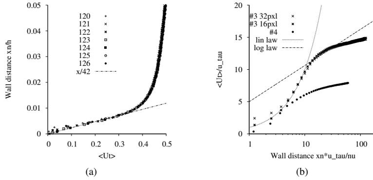
Figure 2: Adjacent profiles of the tangential velocity component at  $x/h = 8$  ( $16 \times 16$  pixels) (a). Profiles of the tangential velocity component, expressed in inner coordinates, compared to the linear law and to the logarithmic law (b).
